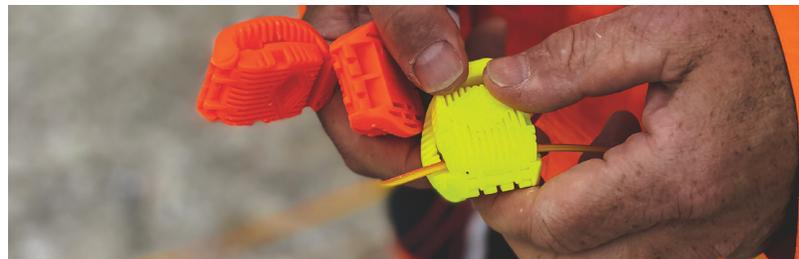
E\*STAR Detonators are equipped with connectors that are weather-resistant, rugged, and easy to open with one hand.
